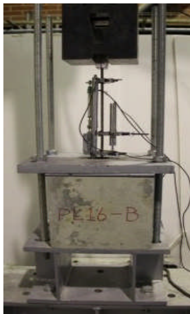
Figure B-3 Test setup for pull-out tests.
