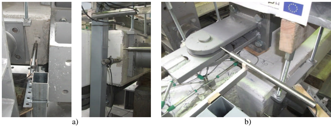
Figure 3-17 Monitoring that can be a source of error: a) Rotation of the foundation in column specimens; b) Rotation of the rods and frame connection at the column-foundation interface.
