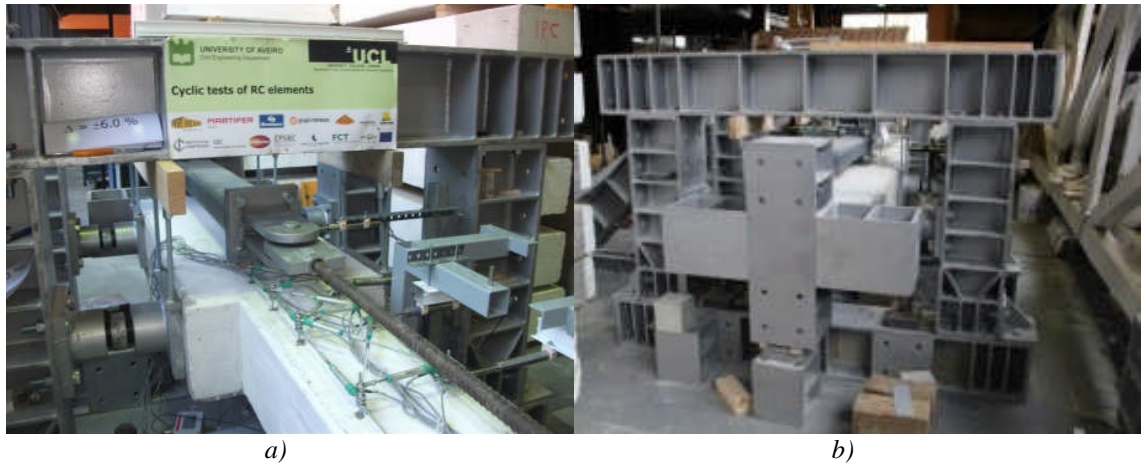
Figure 3-5 Detail of the restraint of the foundation and hinging of the rods: a) from the front; b) from behind.
