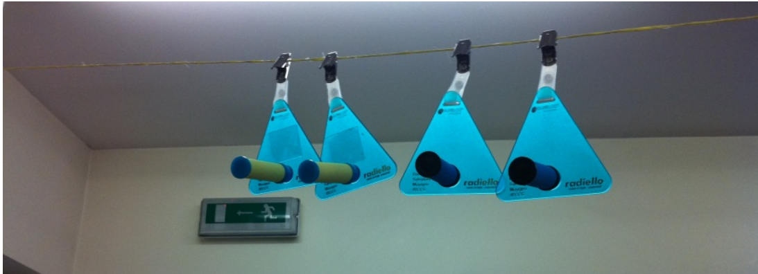
Figure 3.12: Passive diffusive VOC and formaldehyde samplers installed in duplicates in a classroom
