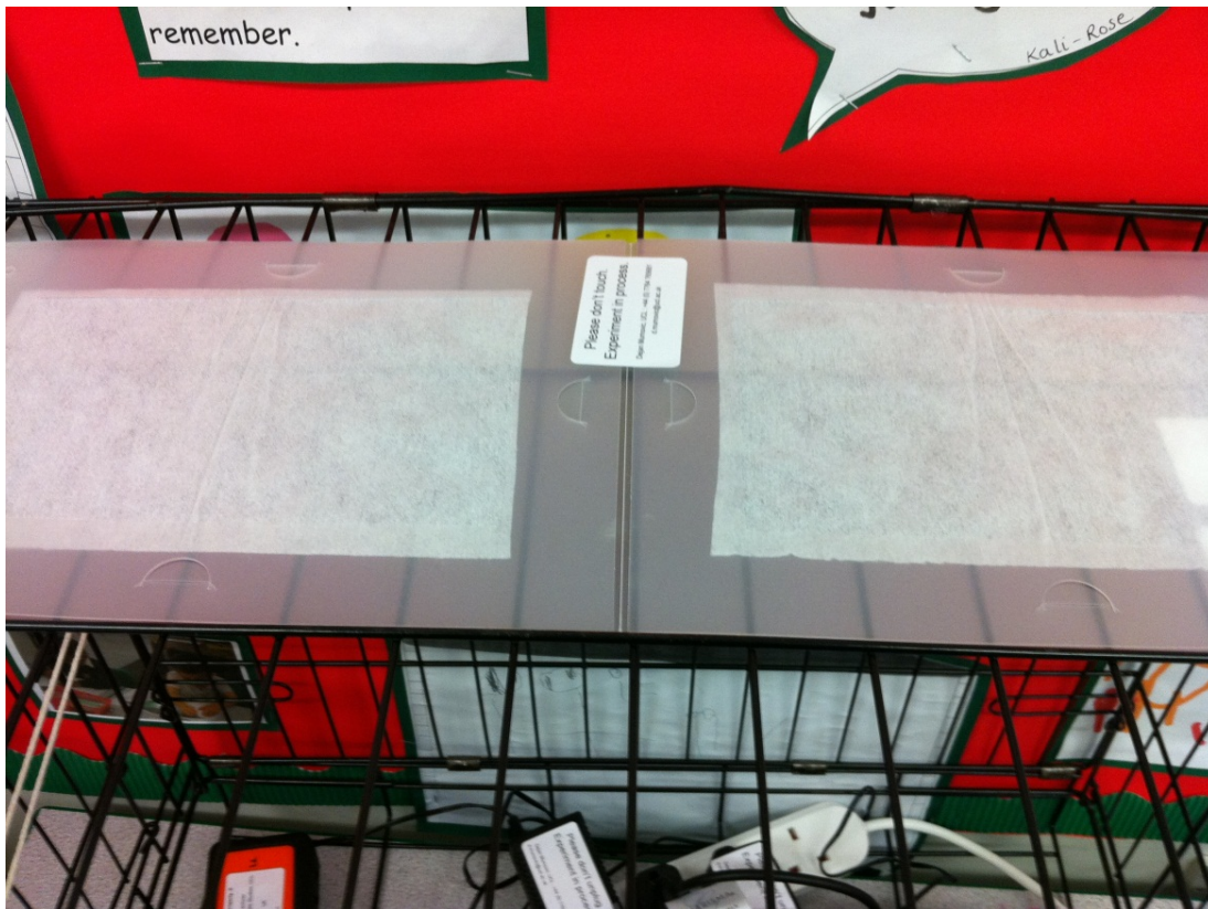
Figure 3.16: Electrostatic Dustfall Collector installed in a school
