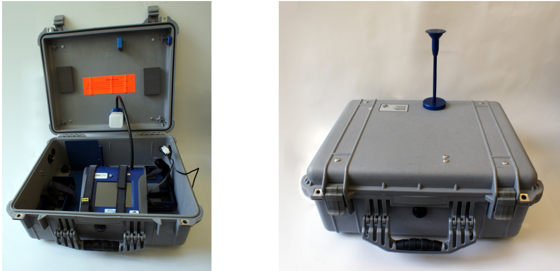
Figure 3.4: Environmental enclosure for laser Particulate Matter photometer
