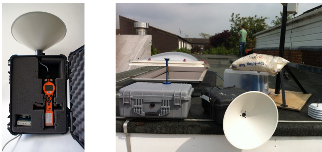
Figure 3.11: External installation for TVOCs detector
