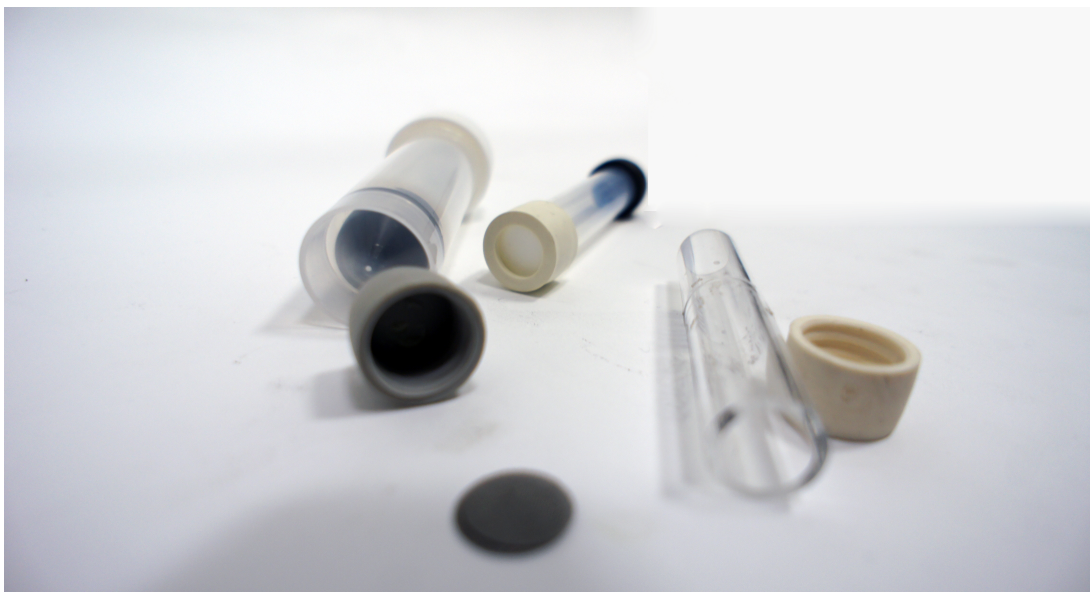
Figure 3.9: Palmes' type tubes for the passive diffusive sampling of ozone and nitrogen dioxide
