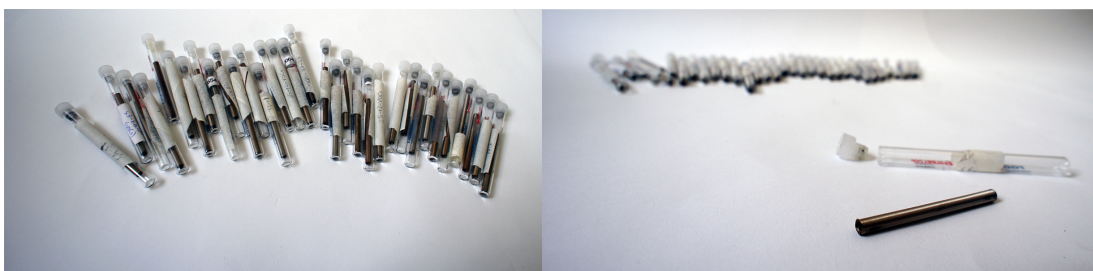
Figure 3.14: Adsorbing cartridges stored in labelled glass vials
