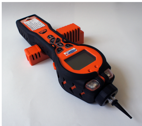
Figure 3.10: Direct reading Photo-Ionisation Detector for continuous monitoring of TVOCs
