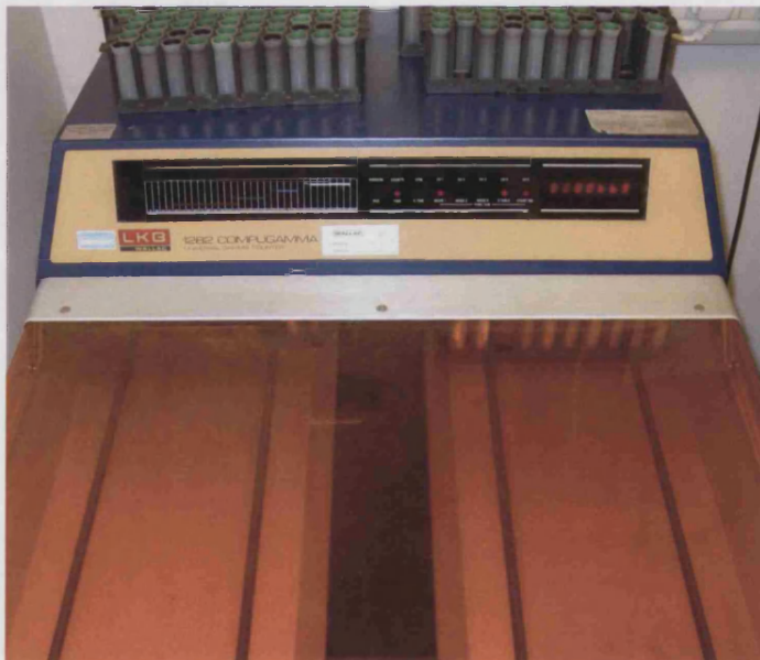
Figure 3.3 Gamma counter (1282 Compugamma, Universal Gamma counter, Wallac, Crownhill, Milton Keynes, UK.)
