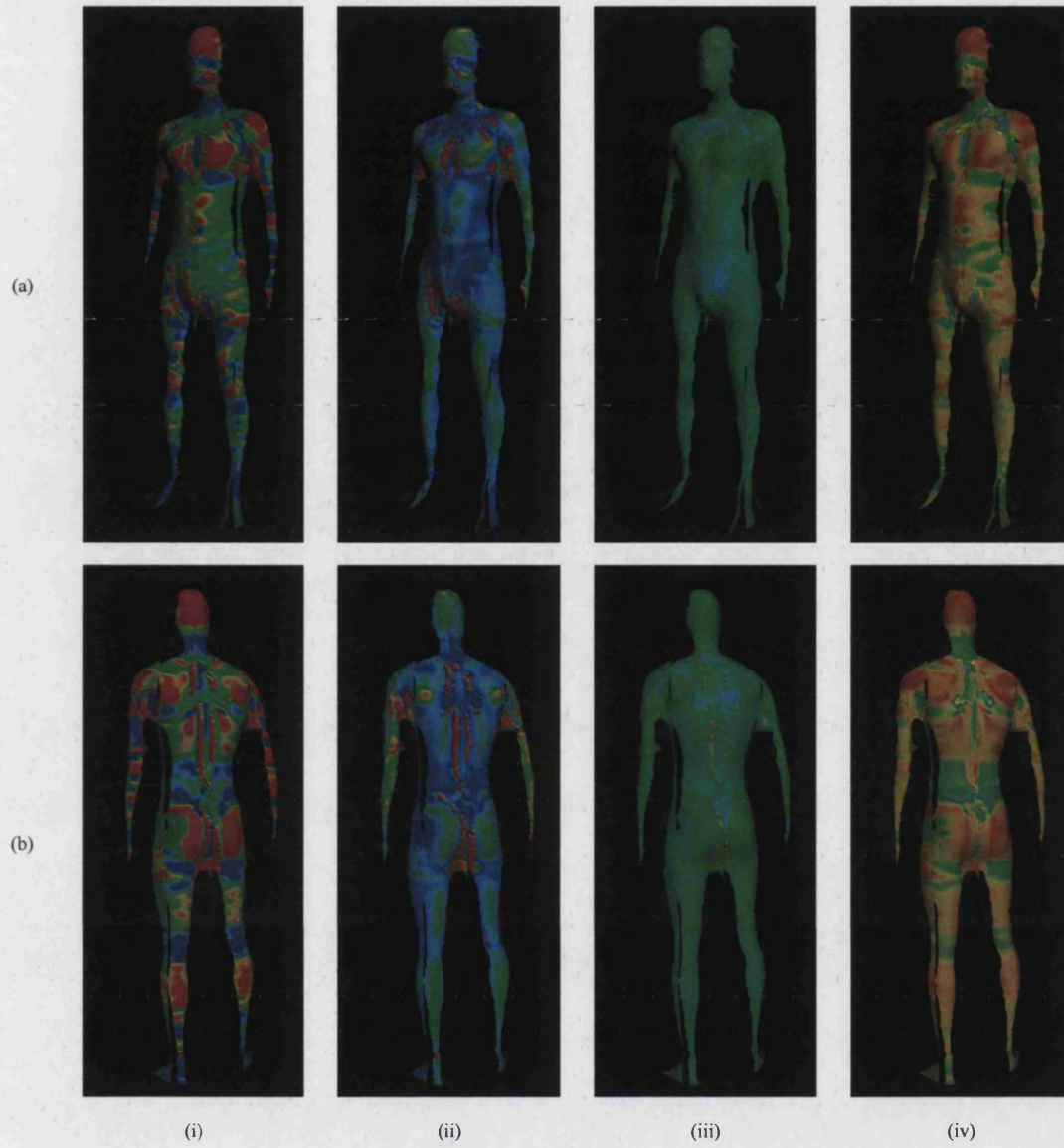
Figure 40: Results for a whole body Hamamatsu scan of a male subject. By row: (a) front view, (b) rear view. By column: Gaussian curvature, mean curvature, curvedness, shape index.
