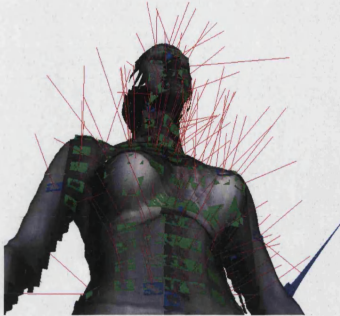
Figure 3: Fitting conic sections to body scanner data using the 3D extension of the method described in [Book79] (green: quadratic patch, blue: cubic patch – red lines illustrate the local surface normals calculated from the patches.). The poor quality of the result is evident when the data set corresponds to a synclastic (elliptic) shape.
