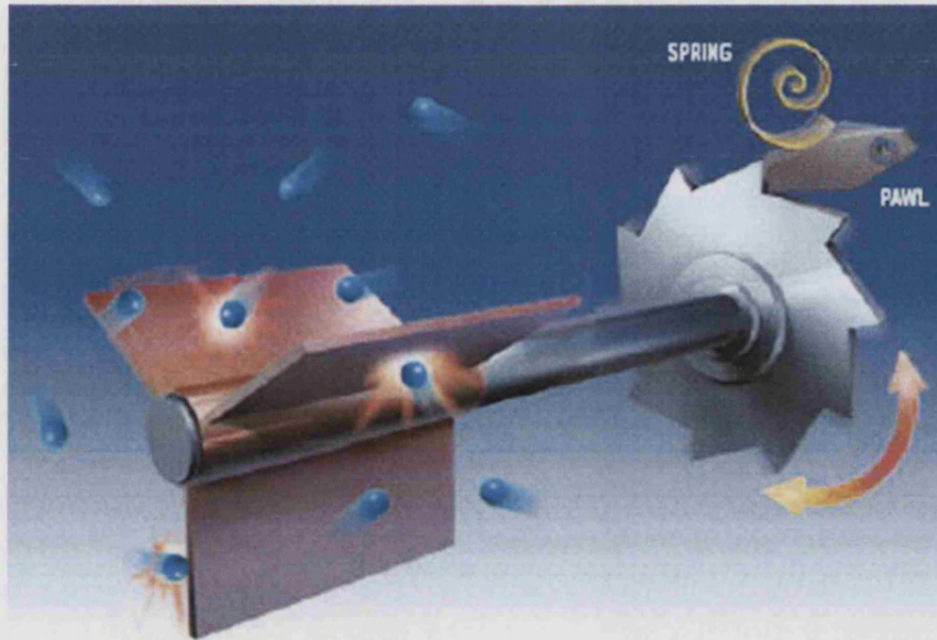
Figure 3.1: A graphical representation of the Feynman ratchet showing both the bombarded panels and the ratchet and pawl. From [50].
