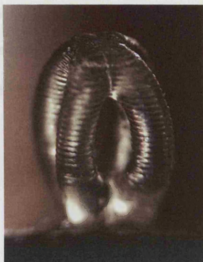
Figure 7.1. Implant (ca. 4x 6 mm) produced with P17L4DMA and the photoinitiator Irgacure 651 TM (2,2-dimethoxy-2-phenylacetophenone) after exposure to UV light at 325 nm using stereolithography. (Courtesy of Dr. Alexander Evseev and Dr. Michail Markov at Institute of Laser and Information Technologies, Russian Academy of Sciences, Moscow).
