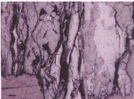
Figure 5.69 Reflected light microphotograph of sample FOU40 (scale 100 μm), showing the edge of the sample with copper minerals.
