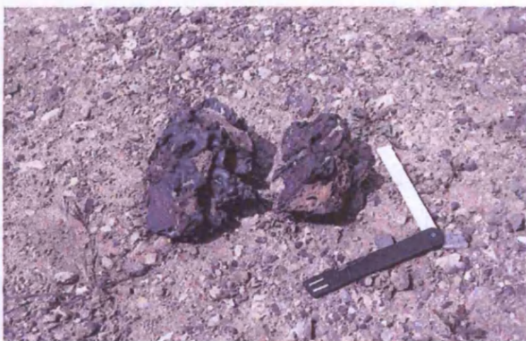
Figure 5.79 Slags from Avessalos bearing large inclusions of schist and ceramic.
