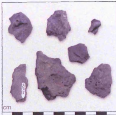
Figure 6.5 Examples of Group 1 slags (top from left: KKN1, KKN4, KKN5; middle: KK1; bottom from left: KKN8, KKN9, KKN10).
