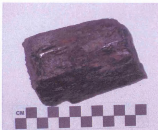
Figure 5.8 Example of dense crystalline slag (sample KEF23).
