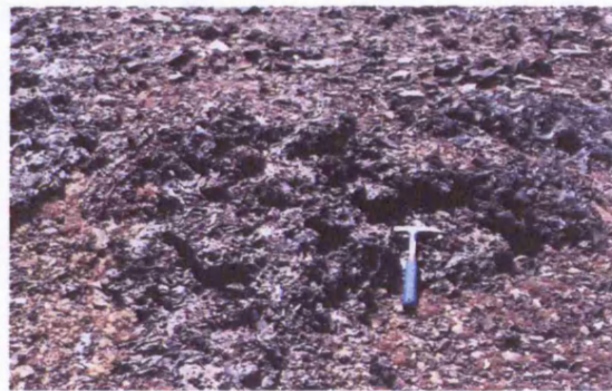
Figure 5.6 Large masses of slag with flow texture at Kephala 1.
