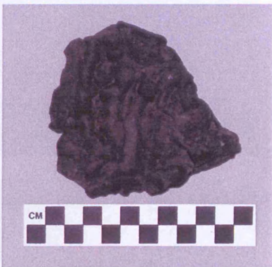
Figure 5.7 Example of slag showing flow texture (sample KEF31).
