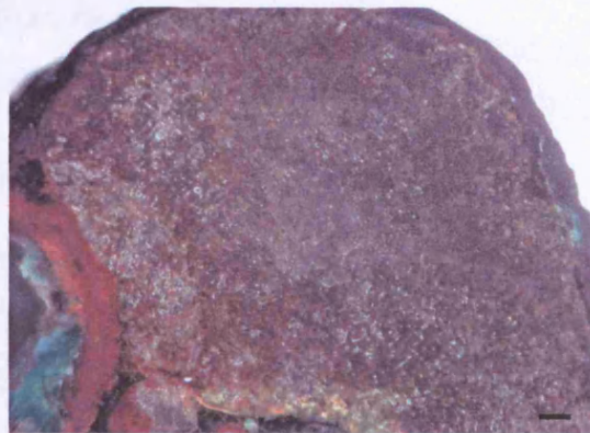
Figure 6.19 Reflected light microphotograph (crossed polars) of completely corroded prill at the edge of sample KKN2 (scale 100 \mu\text{m} ), which retains original as-cast dendritic microstructure.
