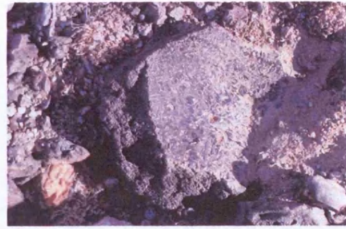
Figure 5.18 Bowl-shaped crystalline slag from Kephala 2 (cut sample KEF10).
