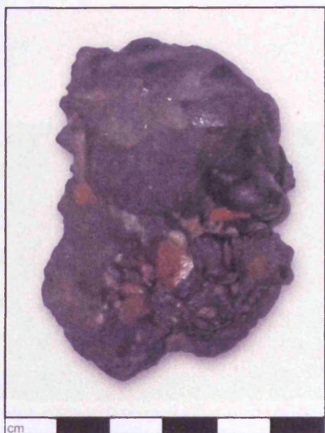
Figure 5.26 Slag sample KEF14 bearing small ceramic fragments on its exterior.
