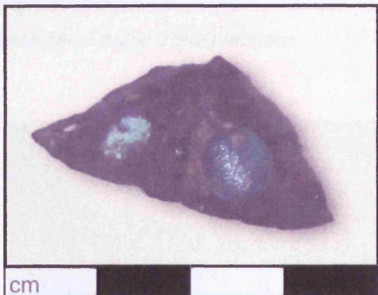
Figure 5.34 Sample KEF40 bearing two external green prills.
