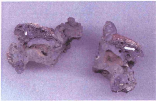
Figure 5.55 Sample FOU22 cut in two, showing enclosed ceramic
