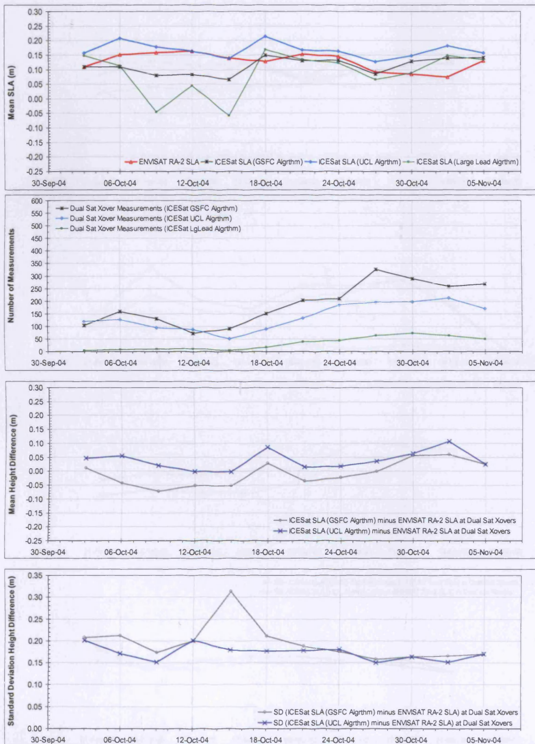
Figure 5.10 L3a campaign 3-day SLA dual-satellite crossover statistics. (First panel) 3-day mean SLA at dual-satellite crossover locations. (Second panel) Number of measurements included in the 3-day mean SLA calculations. (Third panel) 3-day mean crossover height difference (ICESat - ENVISAT) at dual-satellite crossover locations. (Fourth panel) Standard deviation of dual-satellite crossover height differences for each 3-day period.
