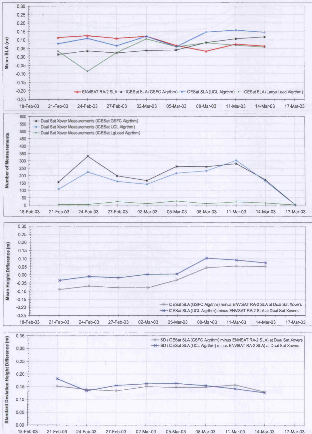
Figure 5.11 L1 campaign 3-day SLA dual-satellite crossover statistics. (First panel) 3-day mean SLA at dual-satellite crossover locations. (Second panel) Number of measurements included in the 3-day mean SLA calculations. (Third panel) 3-day mean crossover height difference (ICESat - ENVISAT) at dual-satellite crossover locations. (Fourth panel) Standard deviation of dual-satellite crossover height differences for each 3-day period.
