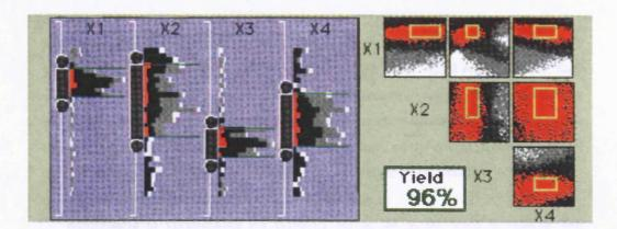
Fig. 2.10: Dynamic interaction with mathematical models to explore manufacturing tolerances (X1 – X4). Optimum yields are displayed within the yellow boxes. (Tweedie, et al., 1994).
