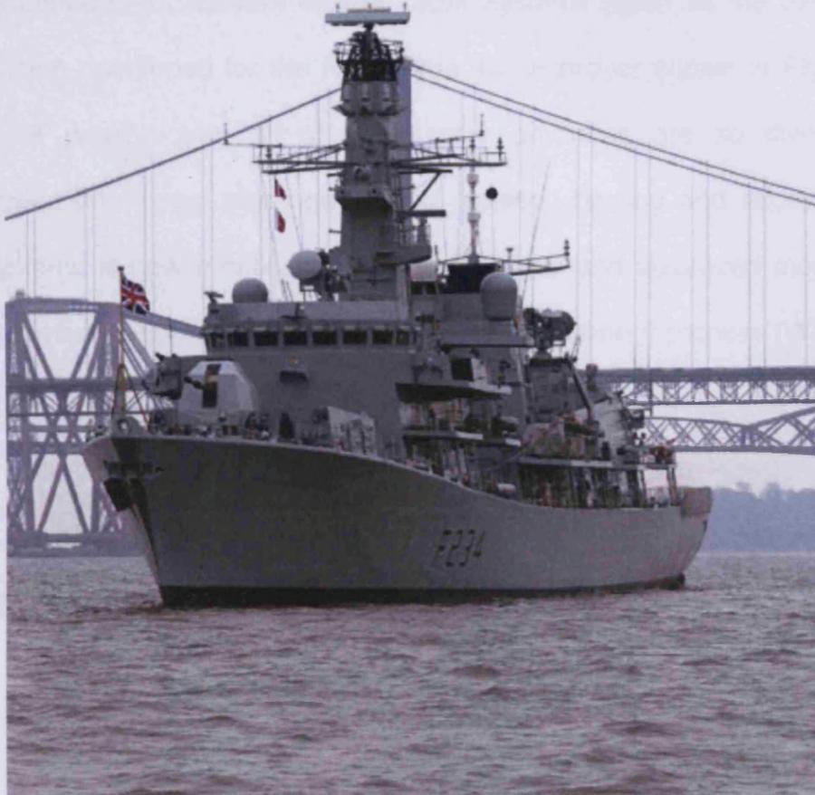
*Figure 1-5 The Type 23 Frigate carries four different radar systems including the T996 radar atop its main mast*
