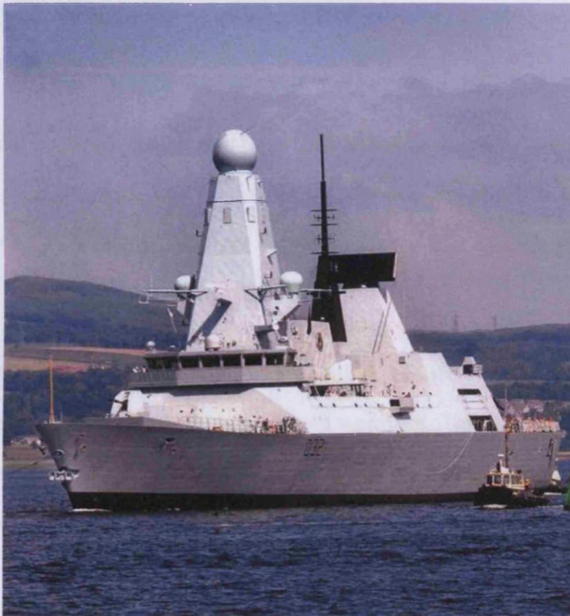
*Figure 1-6 Type 45 Destroyer HMS Daring showing off her egg-like SAMPSON radar during sea trials*
