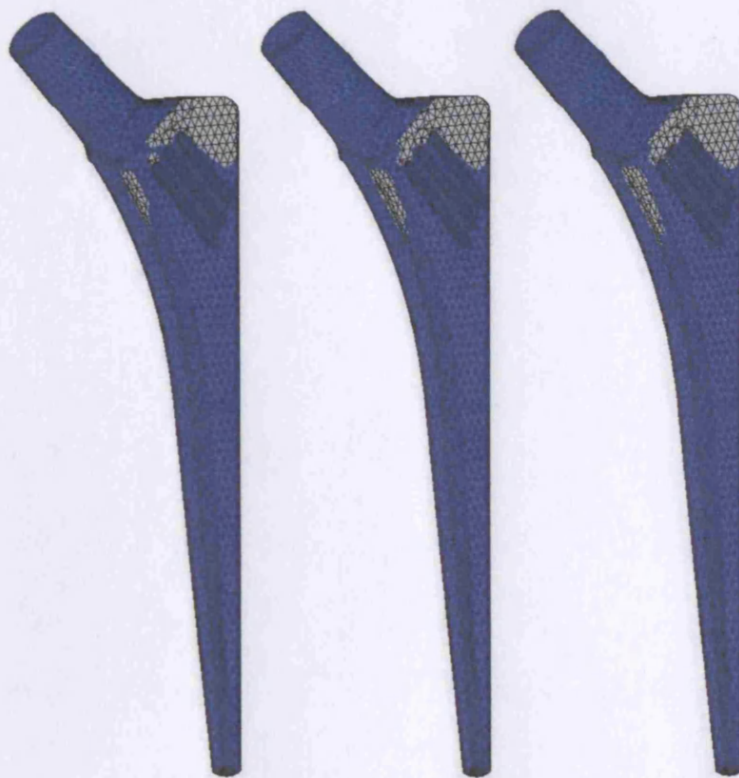
Figure 5.92: Progression of surface area unfeasible for bone ingrowth (grey area) for the 45° grooved CLS under simulated stair-climbing loads (iteration 1 to 3).
