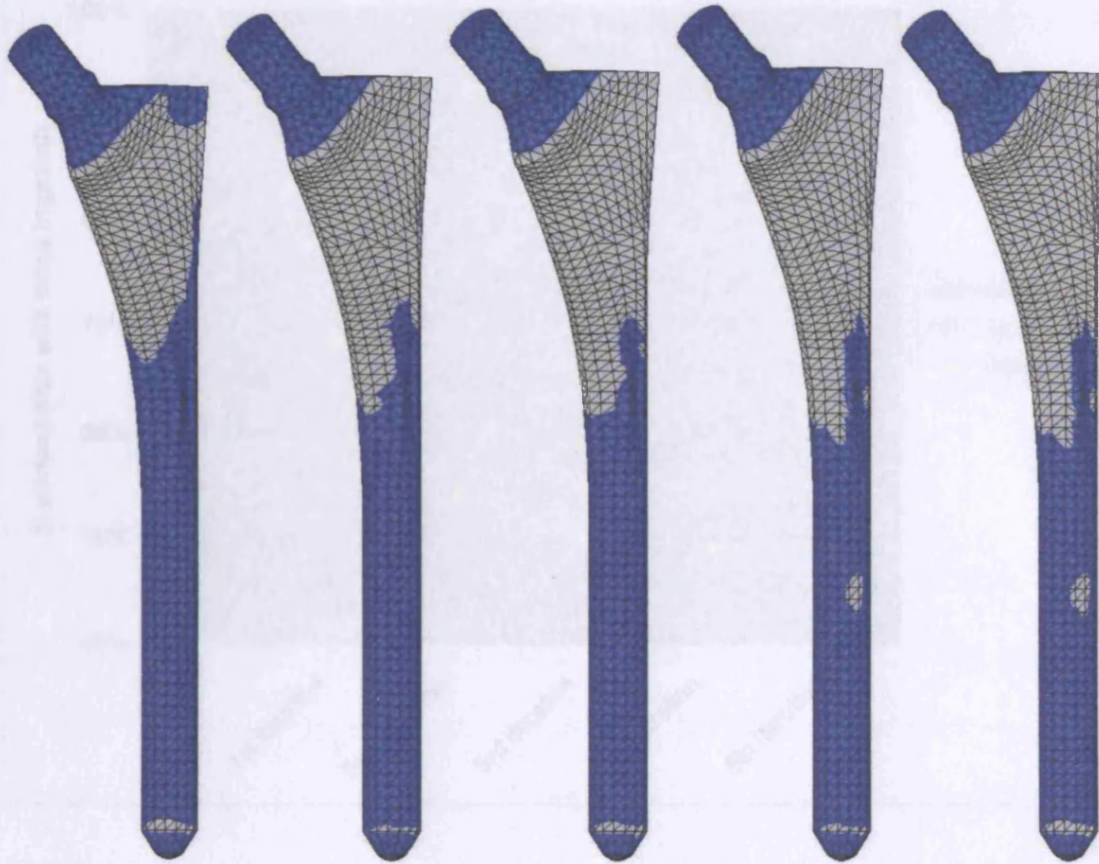
Figure 5.74: Progression of surface area (grey colour) unfeasible for bone growth for the composite stem (iteration 1 to 5).
