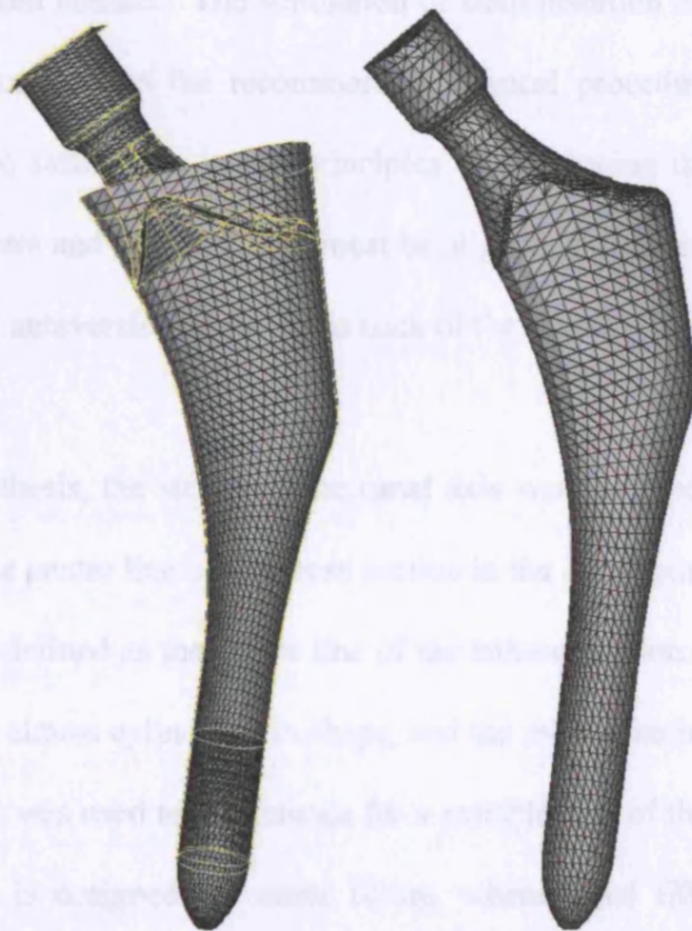
Figure 2.17: The ABG hip stem in the original IGES format surface meshed in MARC (left) and the completed model after repairing the surface boundaries in Magics (right).
