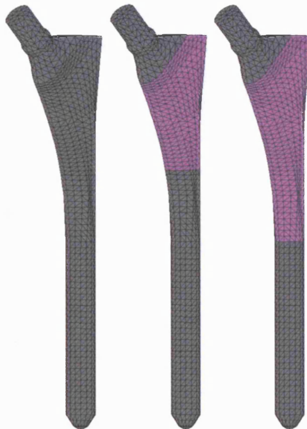
Figure 6.107: Three cases of the AML stem analysed – without interfacial gaps (left), with gaps in the proximal \frac{1}{3} (middle) and with gaps in the proximal \frac{1}{2} (right).
