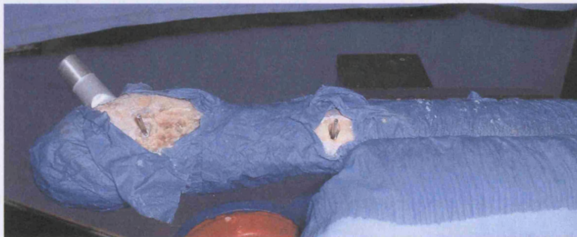
Figure 3.38: Location of the two \phi 2\text{mm} steel pins for micromotion measurement.
