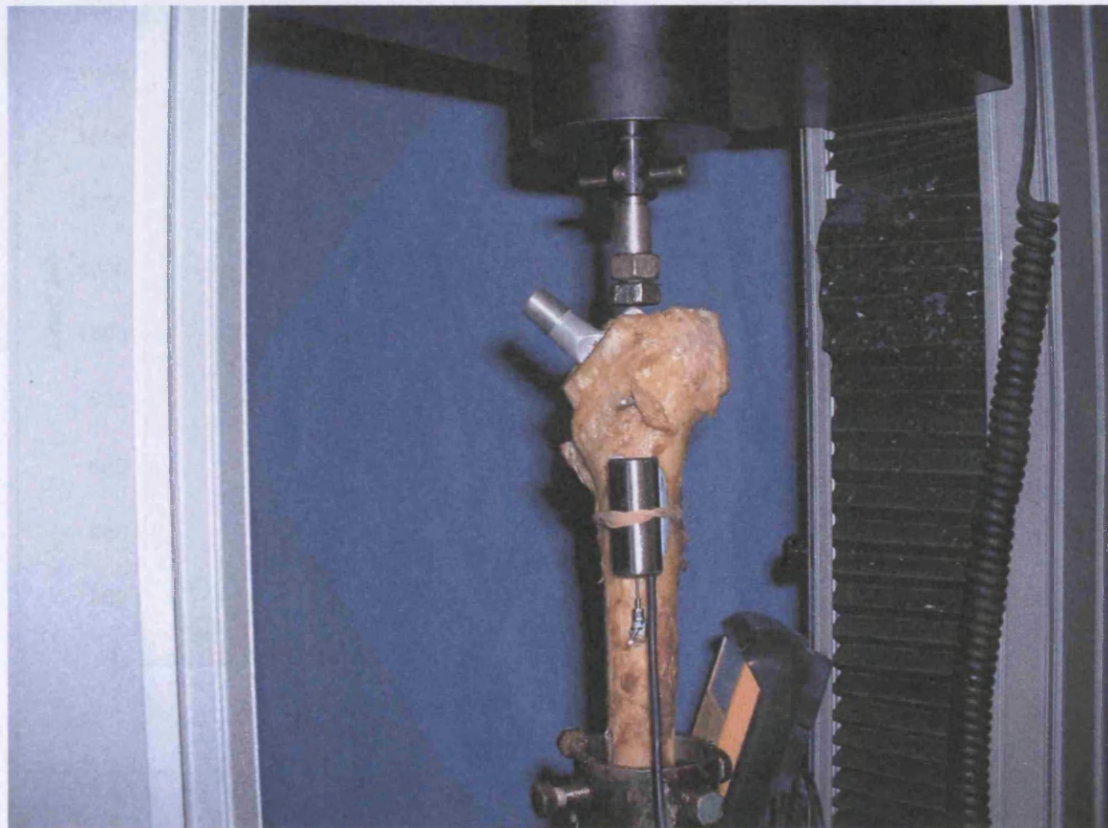
Figure 3.39: The implant loaded in compression using the Instron machine.
