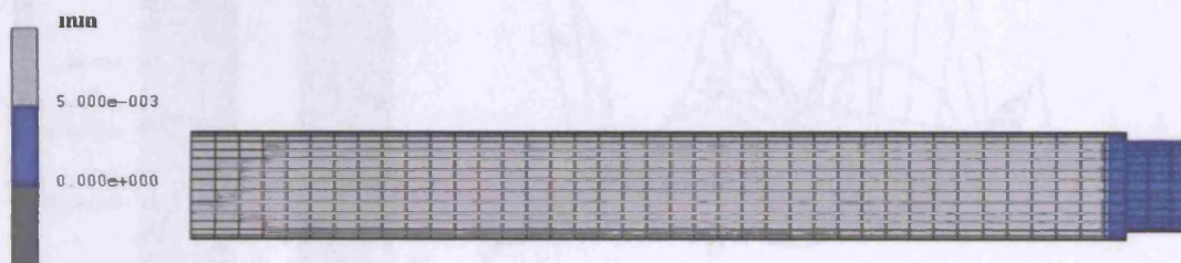
Figure 2.29: Contour plot showing relative micromotion of 5\mu\text{m} when the prosthetic stem (with the coating) was displaced longitudinally by 4\mu\text{m} and rotationally by 3\mu\text{m} .
