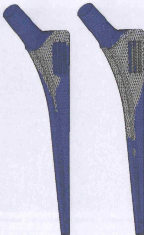
Figure 5.95: Progression of surface area unfeasible for bone ingrowth (grey area) for the vertically grooved CLS under simulated walking loads (iteration 1 and 2).
