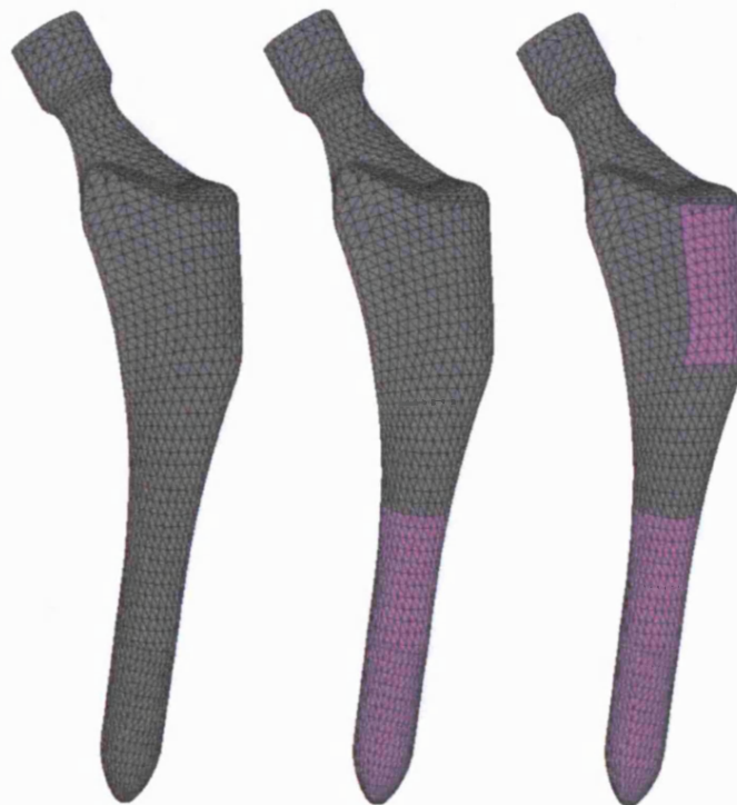
Figure 6.106: Three cases of the ABG stem analysed – without interfacial gaps (left), distal gap (centre) and distal & lateral-proximal gap (right).
