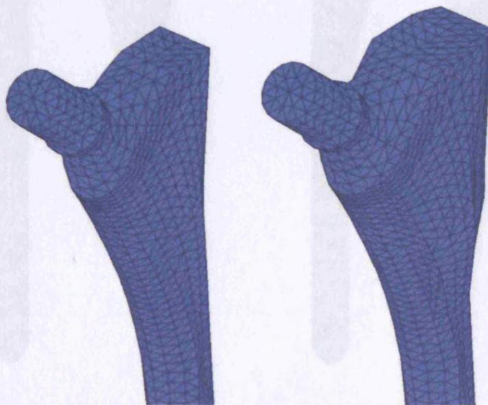
Figure 5.79: The distal fixation design (left) and the proximal fixation design showing enlargement in medio-lateral and antero-posterior directions (right).
