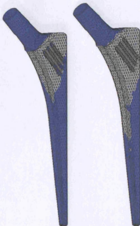
Figure 5.93: Progression of surface area unfeasible for bone ingrowth (grey area) for the 45° grooved CLS under simulated walking loads (iteration 1 and 2).
