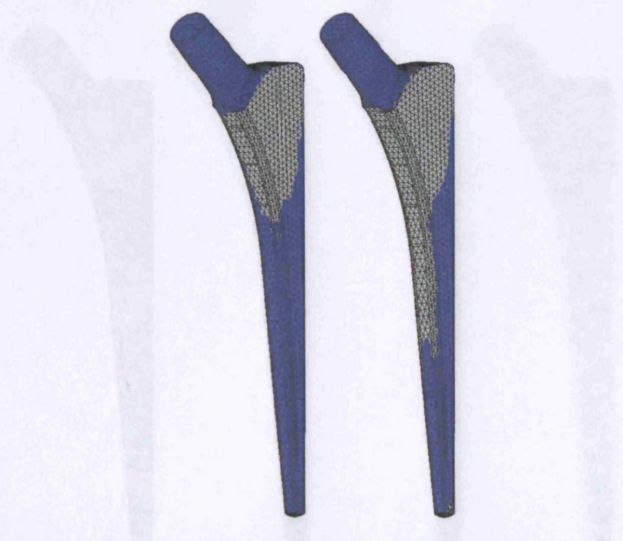
Figure 5.89: Progression of surface area unfeasible for bone ingrowth (grey area) for the blank CLS under simulated walking loads (iteration 1 and 2).
