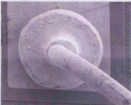
Figure 3.6. Showing electron micrographs, schematic and photograph of the anode section (top left), schematic of completed device (top right), bond pad (bottom left), and completed package (bottom right).
