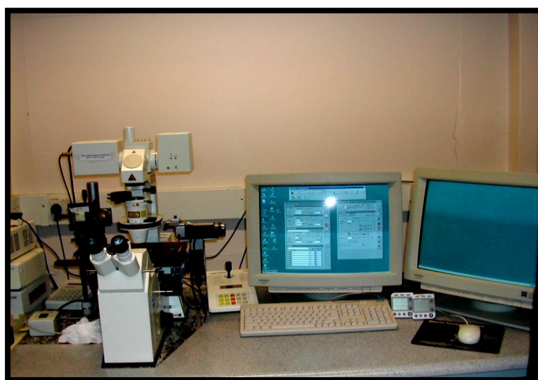
Figure 3-4: Confocal Microscope with Camera Attached
