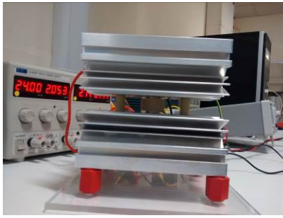
Fig. 25: Double side cooling assembly of the press-pack diode
