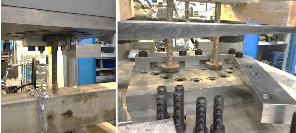
Figure 8: Top reaction plates (left) and bottom reaction plates (right)
