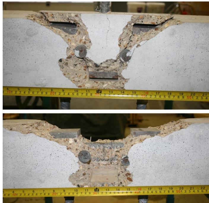
Figure 17: Typical specimen after removal of loose concrete (top) and central headed bar (bottom)
