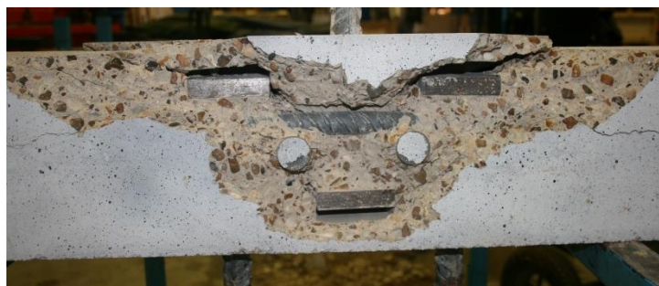
Figure 20: Specimen G3-28-2H20T'B'-S-100-200 after removal of loose concrete
