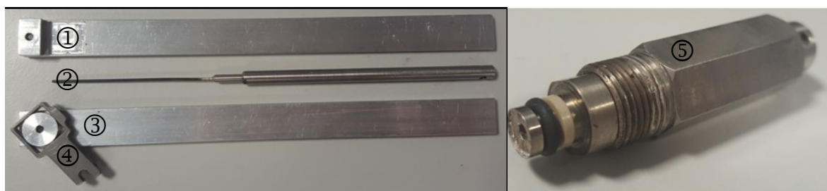
Figure 4.6 Substrate adjuster kit: ① Substrate installation tool, ② extended M2 Allen Key, ③ substrate holder installation tool, ④ substrate holder, ⑤ substrate adjuster port plug.
