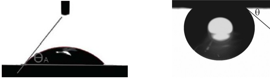
Figure 2.10 Left. Image of a sessile drop for contact angle measurement [52]. Right. Image of a captive bubble for contact angle measurement [53].
