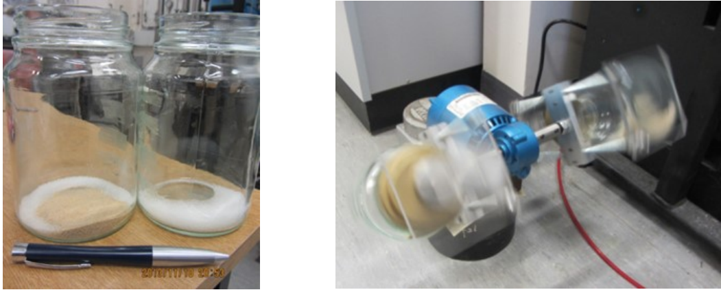
Figure 3.6. Ballotini and Toyoura sand inside jars (left) and milling machine (right).
