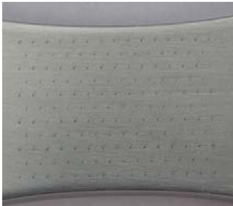
Figure 3 The staggered nature of the array of the laser induced notches which can initiate fatigue crack(s).
