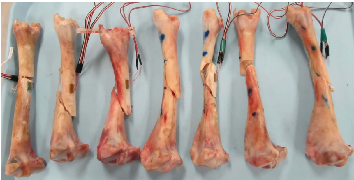
Figure 5.14: Fractured bones from the fast (first three) and the medium groups. The middle two dots in each bone marked the region of constant bending moment in four-point bending. All oblique fractures occurred proximally. A transverse fracture that later progressed into a butterfly fracture can be seen in the third bone from the right.
