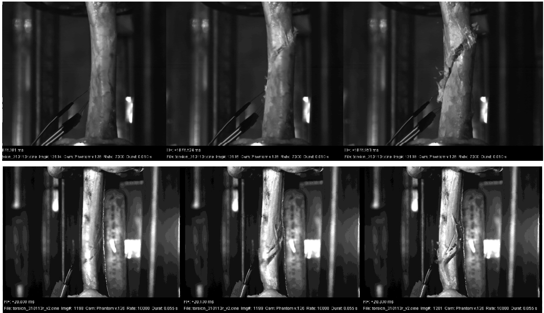
Figure 5.19: (Top) The fracture progression of a 'clean' spiral that took place over 0.572ms in three video frames (frame rate of 7000 fps) for a tibia tested at the low strain rate (TS4). (Bottom) The fracture progression of spiral fractures with several fracture paths (TF4) acquired at 10 000 fps.
