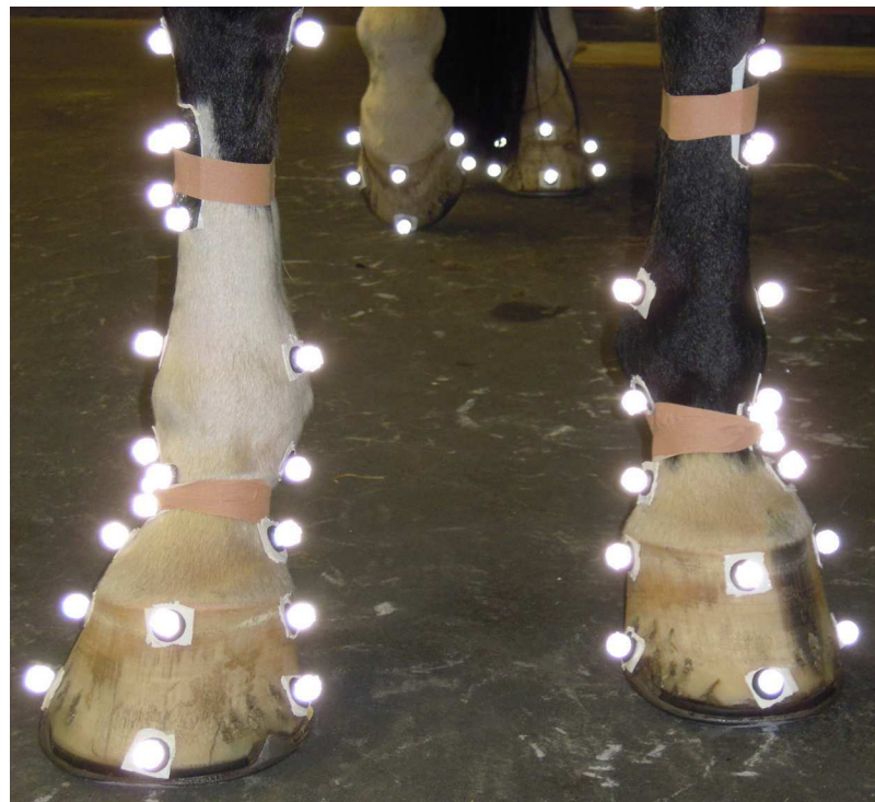
Fig 1. Marker setup of both limbs. Joint centers of the lower limb and 6 markers on each hoof were attached to the horse using sticky tape.
