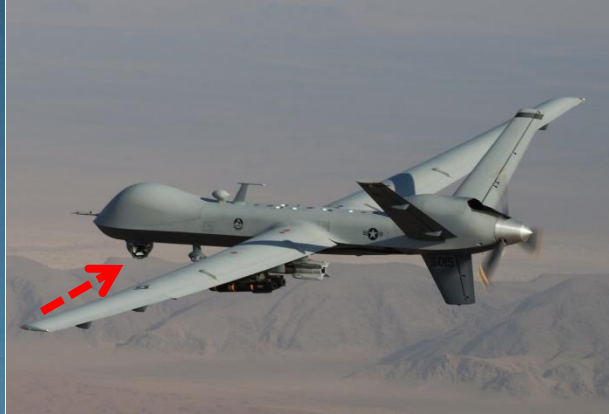
Figure 2: USAF MQ-9 Reaper Aircraft [8] Sensor camera location highlighted.
