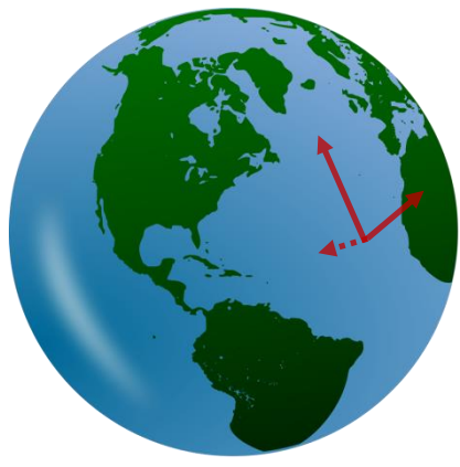
Figure 6: Earth Axis System This axis is oriented north, east, and down into the earth.
