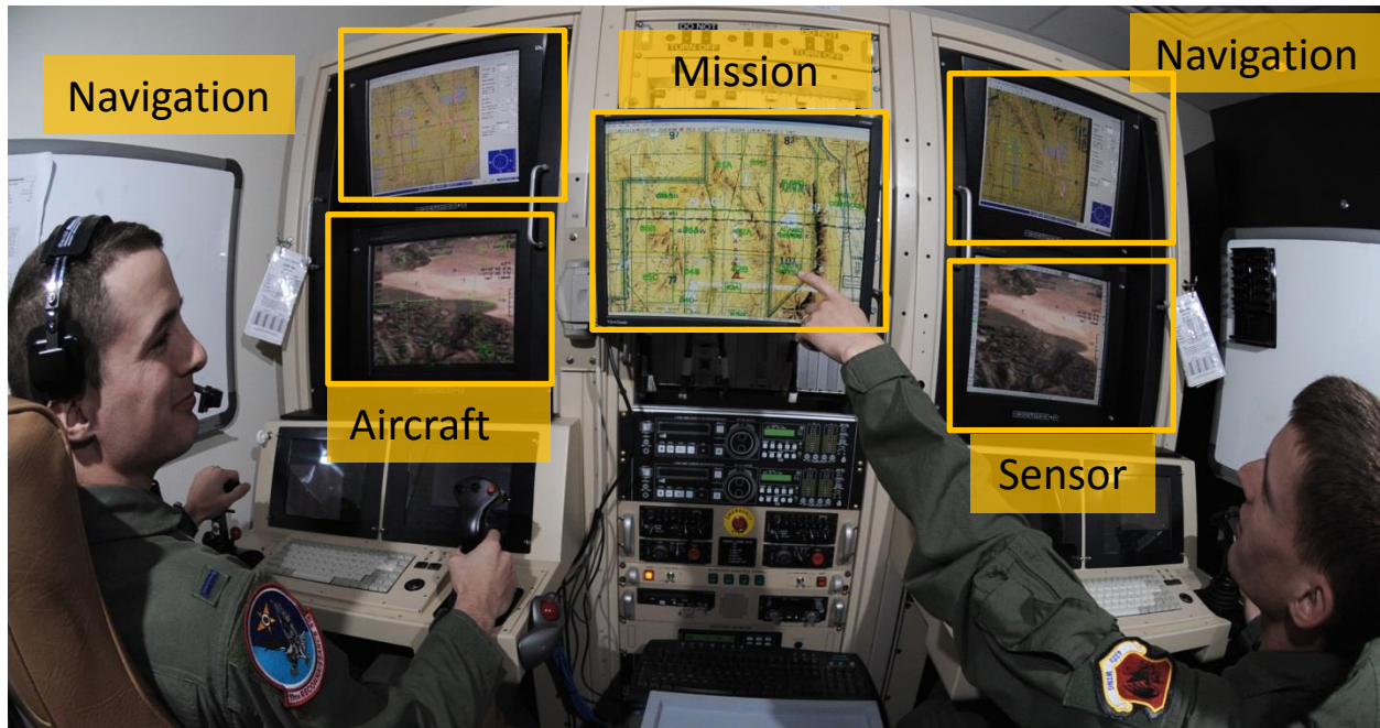
Figure 3: USAF MQ-1B Predator Control Station [55]
