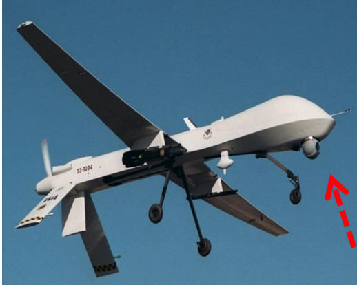
Figure 1: USAF MQ-1B Predator Aircraft [9] Sensor camera location highlighted.
