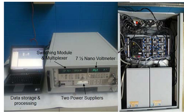
Fig. 3 Photograph of electronic components of ESAP-DCPD system
