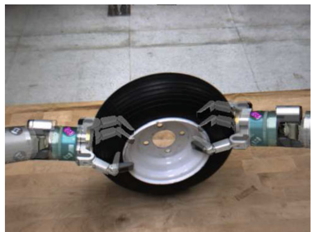
Fig. 7 Two fiducials detected shown in red and the overlaid estimated robot location
