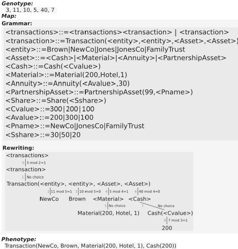
Fig. 3 Example of a mapping from genotype to phenotype through a grammar. An integer string is converted into a transaction between the entities ‘NewCo’ and ‘Brown’ in which Brown gives Cash to NewCo in exchange for a Hotel
