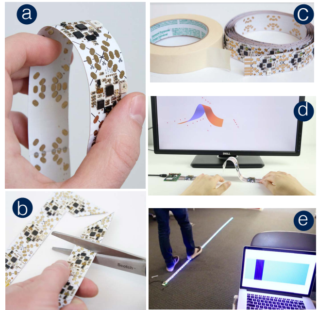
Figure 1. a) Current flexible circuit prototype, showing electronics of two nodes. Each node has a microcontroller, inertial measurement unit (IMU), proximity and light sensors. b) SensorTape can be cut anywhere and rejoined. We develop algorithms to automatically determine the order and the number of nodes. c) Form factor of SensorTape is of 1-inch wide masking tape. d) SensorTape sensing its deformations with IMUs e) The 2.3 meter long testbed with 66 sensor nodes. Proximity sensors are visualized on the laptop, while hovering foot over the tape.
