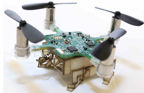
Fig. 1: Our 30g flying monkey. Videos of the experiments conducted are available as a video attachment and at http://mrs1.grasp.upenn.edu/yashm/ICRA2016.mov .
