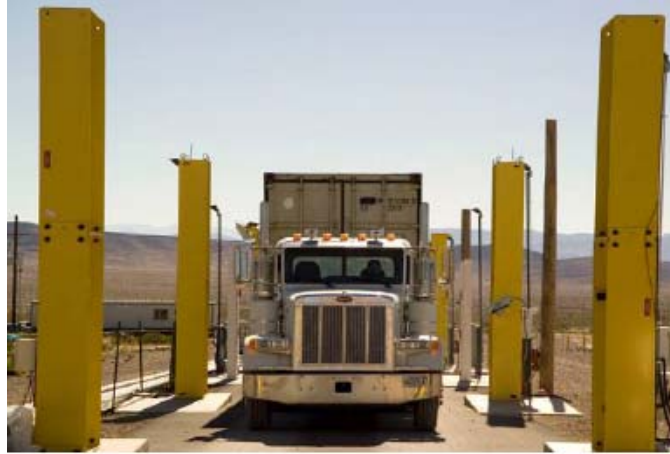
Figure 5: Fixed-site passive radiation portal monitoring 35
