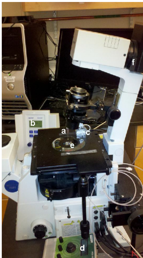
Figure S.1 Experimental setup. Picoliter droplets of aqueous media are delivered using microcapillaries (a) regulated by microinjectors (b). Micromanipulator (c) controlled by joystick (d) enables 3D motion of the microcapillary. The hydration reaction as it unfolds on the glass slide (e) can be observed through the optical microscope (f). Camera attachment of the optical microscope enables storing and subsequent analysis of images on a local computer.
