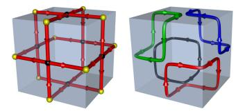
FIG. 1. Structure of L lattice. Left figure: Nodes and links (with associated orientations) in the unit cell of the L lattice. The two sublattices of nodes are indicated. Right figure: One of the four equivalent packings of minimal-length loops on this lattice.
