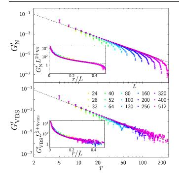
FIG. 9. Derivatives of Néel and VBS correlators,  $dG_{\text{Néel}}(r)/dr$  and  $dG_{\text{VBS}}(r)/dr$ . The main panels show raw data and power-law fits (dashed lines) with  $\eta_{\text{Néel}} = 0.259(6)$  and  $\eta_{\text{VBS}} = 0.25(3)$ . The insets show scaling collapse of  $L^{2+\eta}G'$  versus r/L, with the same values for  $\eta_{\text{Néel,VBS}}$ .
