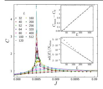
FIG. 6. Main panel: Heat capacity *C* versus *J*. Upper inset: Peak height  $C_{\text{max}}$  with constant  $C_0 = 0.9836$  subtracted to account for background. The fit is the power law with exponent  $\alpha/\nu = 1.52(2)$ . Lower inset: Standard deviation in energy at J = 0.08850. The fit is with exponent  $(\alpha/\nu - 3)/2 = -0.97(4)$ .
