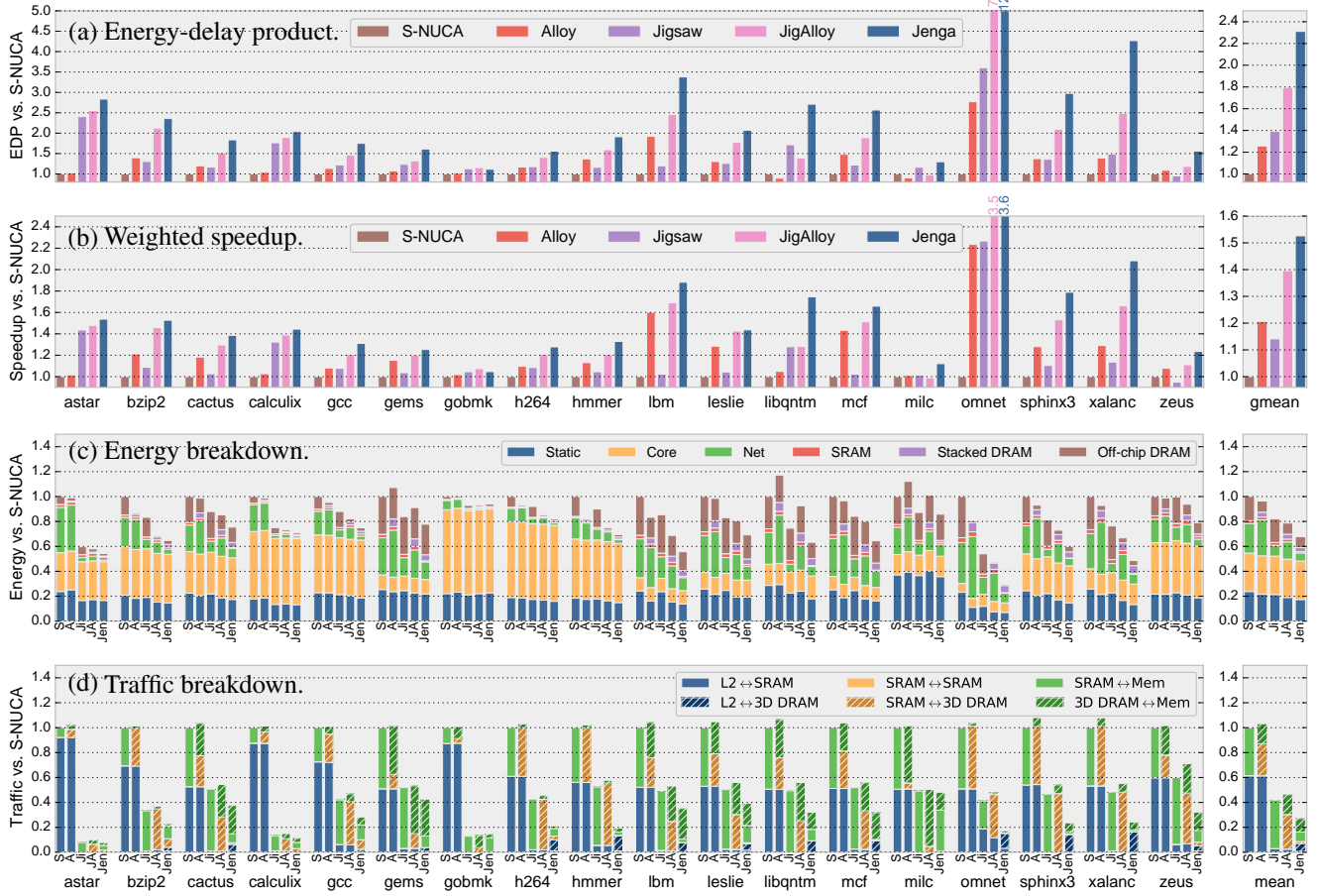
Figure 15: Simulation results on 36 concurrent copies SPEC CPU2006 apps (rate mode).
