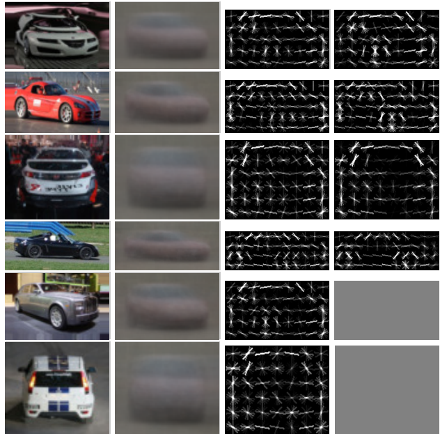
Figure 4. The mixture of root model before and after the training by \ell_1 - \ell_2 norm for the car category. Each row corresponds to a component. First column shows a positive example from the component. Second column shows the average image for the component. Third and fourth columns show the root filter of the component before and after training respectively. A complete gray image indicates the filter is sparse. We can see that the components 4,5 were very similar components 2,3 and thus were removed.
