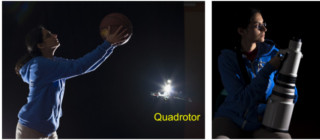
Fig. 10. Left: subject with clothing that is not tight. Right: the subject holding a lens, which caused a strong dominant rim by setting rw_{desired} = 20 , with actual achieved rw_{average} = 17 .
