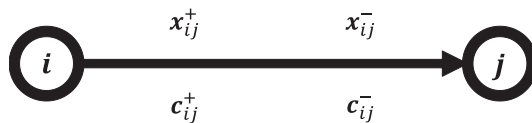
Fig. 3 Outflow x_{ij}^+ , inflow x_{ij}^- , and unit costs for outflow c_{ij}^+ and inflow c_{ij}^- .
