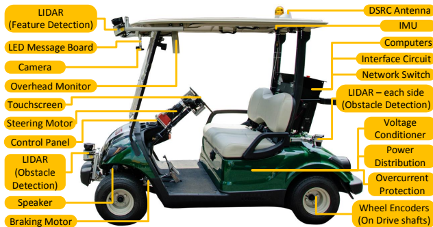
Fig. 1: Hardware overview, highlighting primary retrofit additions to a Yamaha YDREX3 golf car in order to enable autonomous capability.
