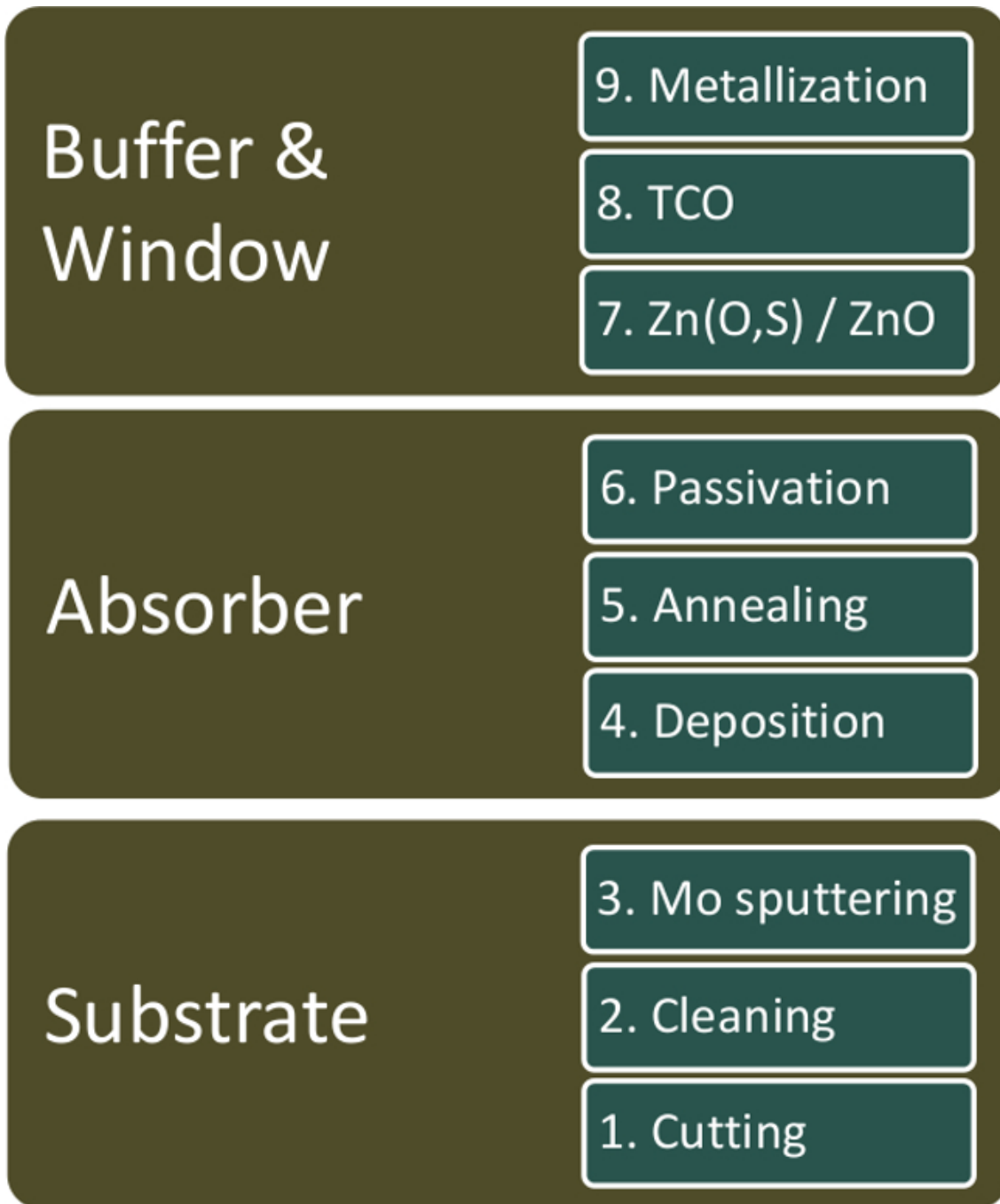
Figure 1. Device fabrication process. Enumeration of the device fabrication process, from substrate cutting (#1, bottom) to metallization (#9, top).
