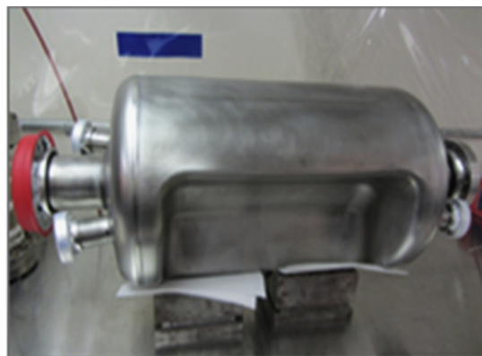
RF-Dipole Nb prototype (Old Dominion Univ., Jlab, SLAC)
