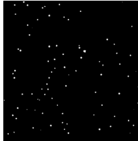
Fig. 8. Large-area optical performance of the OBF. Imager is flood illuminated with uniform light over the CCD and integrated for 20 seconds. Areas where the light is penetrating and visible above the noise floor are shown in white.
