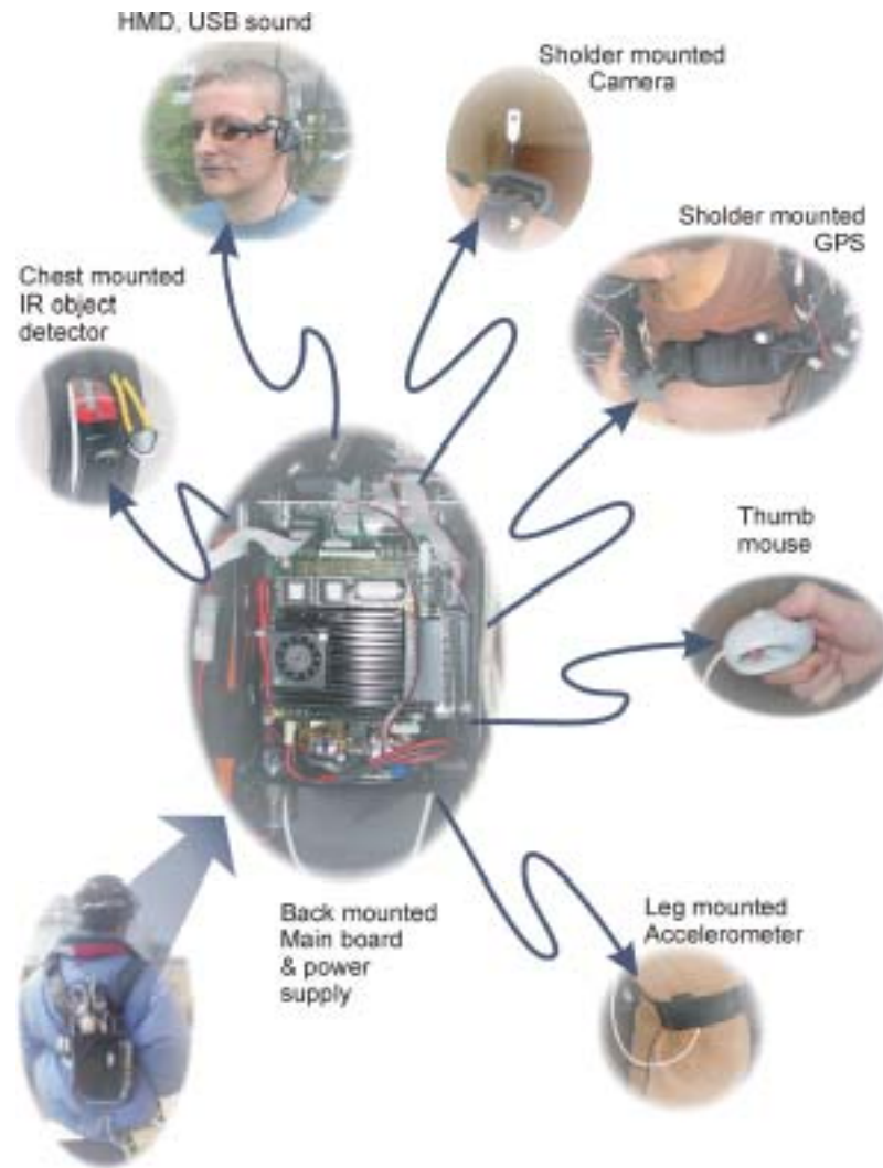
Figure 22 - Components of the final wearable computer
