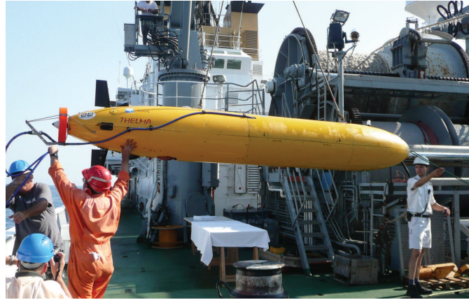
Fig. 3. The NURC OEX-Harpo AUV used during GLINT '10. This AUV communicates with the ship and the MIT Unicorn AUV via acoustic communication (underwater). It also carries a GPS for positioning.
