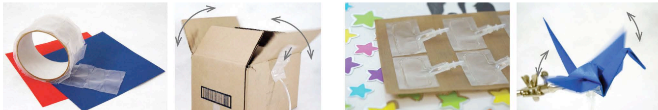
Figure 1. The tape actuator and an active box (left). The sticker actuator and an actuated origami crane (right)
