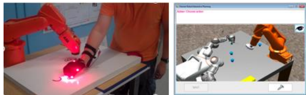
Fig. 1. (Left) Snapshot of human-robot task execution from human subject experiments, (Right) RobotStudio® point-and-click simulation environment for robot training used in our prior investigation.
