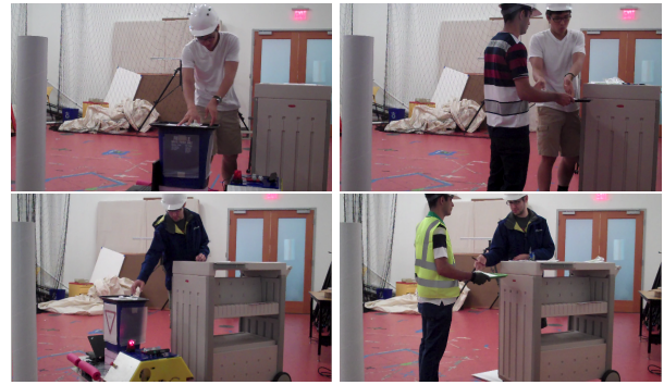
Figure 5: Typical deliveries made by the Assistants (Top row: approach angle = 90^\circ , Bottom row: approach angle = 45^\circ , Left column: robotic assistant, Right column: human assistant)
