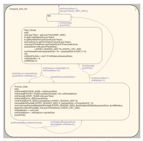
Figure 11 The details of the state machine for the transport layer transmitter controller.
