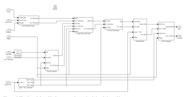
Figure 9 The demodulator block converts the received signals into a bit stream.
