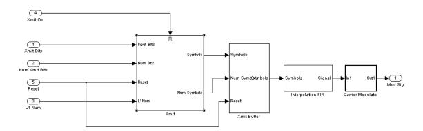
**Figure 4** The modulated symbols are passed through an interpolation filter and carrier modulated before sent to the channel.
