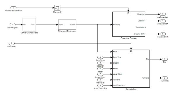
Figure 7 Block diagram of the acoustic receiver.
