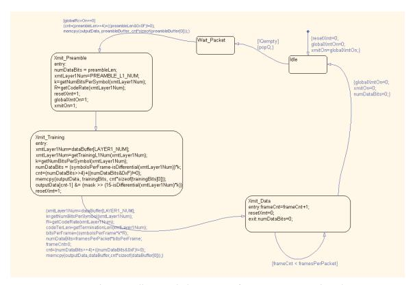
Figure 3 Layer 1 transmitter controller controls the sequence of events to create acoutic packets.
