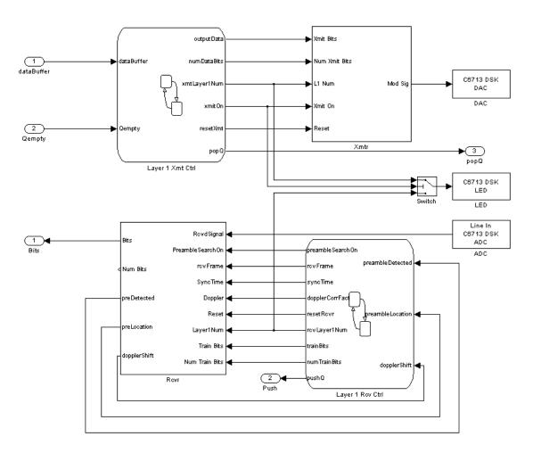
Figure 2 Physical layer (Layer 1) of rModem consists of the transmitter, the receiver, layer 1 controllers, and AD/DA converters.
