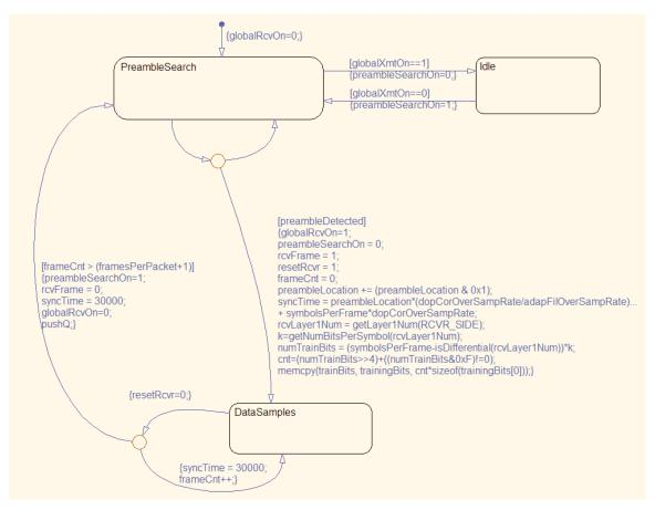
Figure 6 State machine of the physical layer receiver controller handles the operations of the acoustic receiver.
