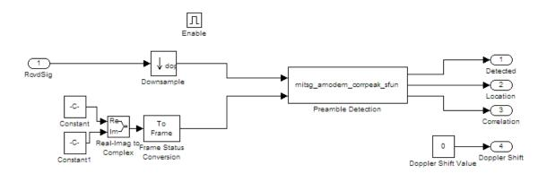
Figure 8 The preamble search block correlates the received samples with the known preamble.
