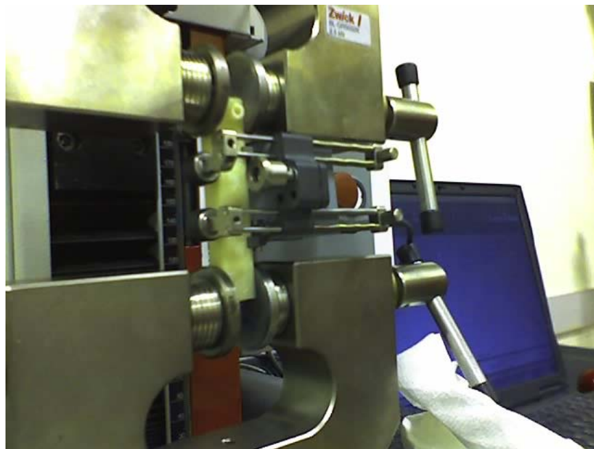
Figure 10: a block of ABS plastic undergoing stress-strain tests in a tensometer.
