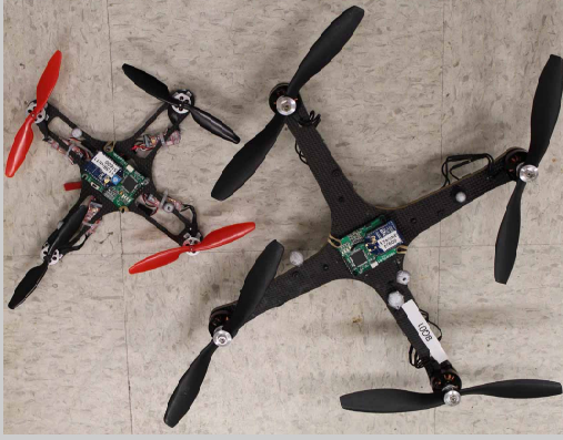
Fig. 1. Two MIT quadrotors equipped to fly in the ACL Real Time Indoor Autonomous Vehicle Test Environment (RAVEN) [40]. The baseline controller on both quadrotors is PID. The gains have been tuned for the bigger quadrotor. The small quadrotor uses gains from the bigger one, resulting in relatively poor trajectory tracking performance.
