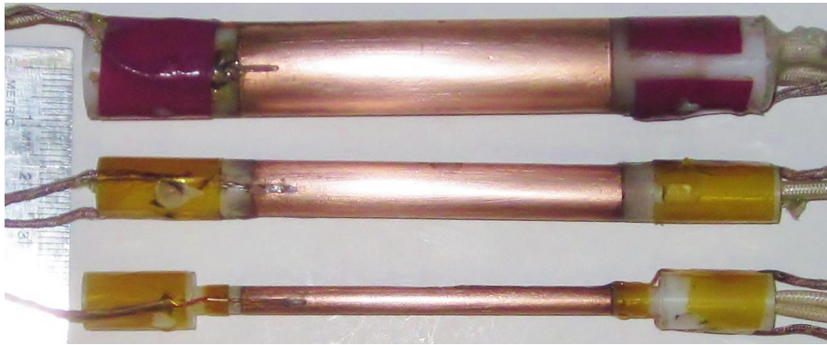
Fig. 1 The three heat transfer coefficient probes
