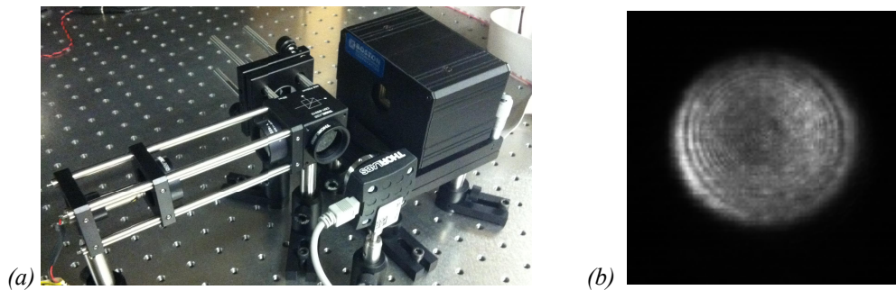
Figure 4: CubeSat-sized MEMS DM Michelson interferometer prototype experiment, initial tip-tilt results. (a) The setup includes a 1.5 micron stroke Boston Micromachines Mini deformable mirror, a Thorlabs CPS180 635 nm 1 mW round beam collimated laser diode module, a cube beam splitter, a pinhole spatial filter, a neutral density filter, a flat mirror, and a Thorlabs DCC1545M \frac{1}{2} " monochrome CMOS camera. A Matlab interface to the mirror driver is commanding the 32 actuators into a “tilt” or “tip”. (b) The interference pattern when the MEMS deformable mirror is set to “flat”.
