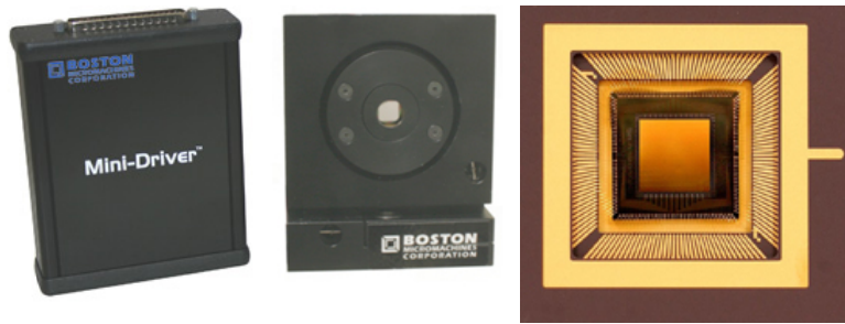
Figure 2: Boston Micromachines Mini 6 \times 6 (32 actuator) deformable mirror and drive electronics[43]. The drive electronics board could be used in a CubeSat without the packaging and with some minor modifications to the board.
