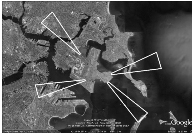
Figure 7: Approach areas for two runways at BOS. Aircraft within the white cones are assumed to be utilizing the runway.
