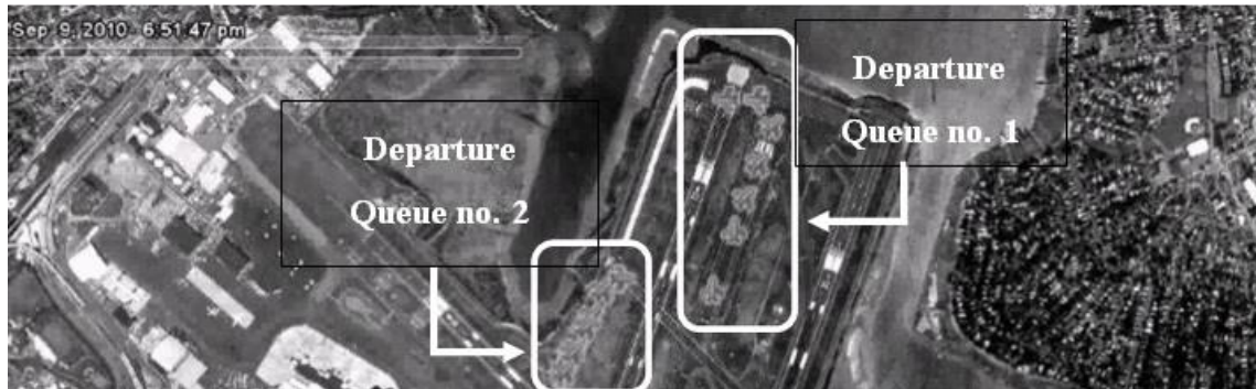
Figure 2: Visualization of queuing behavior at BOS. Aircraft icons represent departing aircraft queuing for departure from Runway 22R. The current queue size is 12 aircraft, with 7 aircraft on the east side and 5 aircraft on the west side of the runway.
