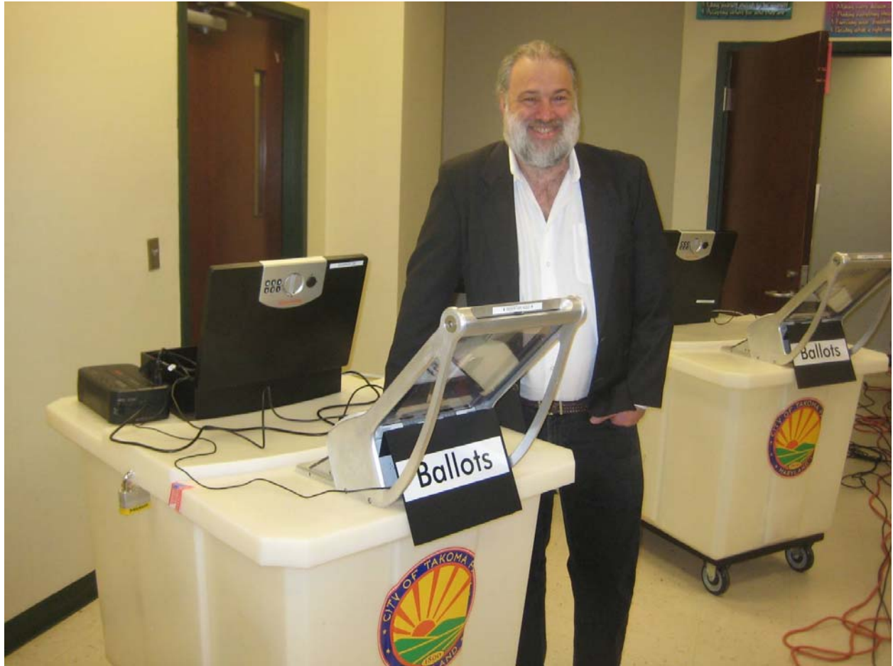
Figure 1. Scantegrity II ballot box / scanner. David Chaum stands beside a Scantegrity II ballot box with attached scanner, as used in the 2009 municipal election at Takoma Park, Maryland. It is impossible for a voter to drop a ballot into the ballot box without scanning it.
