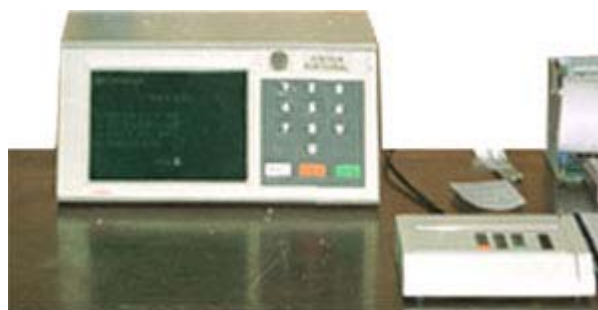
Figure 3-5 – Unisys's Voting Machine Prototype
